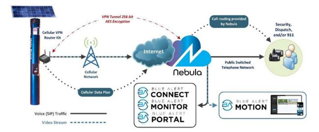
Nebula subscriptions include Code Blue's Managed Services. These services effectively provide system configuration, ongoing support, and proactive monitoring for your emergency speakerphones. The most knowledgeable and experienced technicians deliver a reliable call routing and monitoring system, provide a single source for troubleshooting and updates, implement the most up-to-date software releases, and perform other tasks to maximize your investment.
