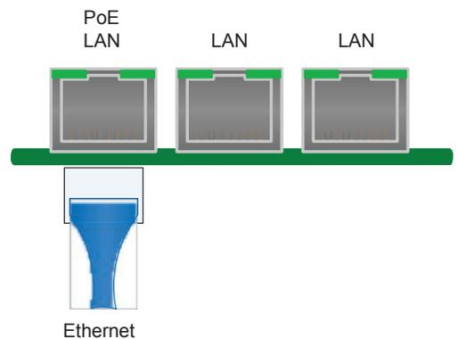
Note that if the IP5000 is configured with a VLAN ID (see section 10, "VLAN Configuration"), only the speakerphone itself will communicate using VLAN-tagged packets. If additional devices connected to the IP5000's other Ethernet ports must communicate on a VLAN, they must either support VLAN tagging themselves (which will be passed through the IP5000's built-in switch) or the upstream connection must be providing untagged packets from that VLAN.
