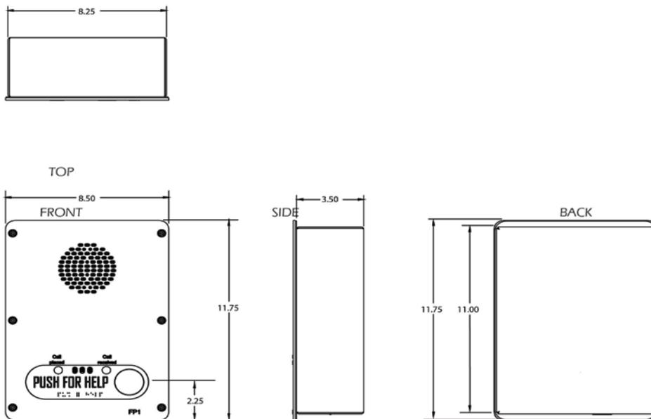
**NOTE: mounting holes and conduit hole by others**
